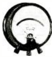
Model 525 D. C. Portable Accuracy within 1%
